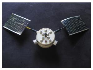
with 1 milliwatt or less of power. The networking capabilities happen over a local X-Bee network, giving the instruments the capability of group synthesis. This project is still in progress, but so far has resulted in promising results. Shown here is the first working prototype, which also is able to broadcast its sound over a low-power FM transmitter. The hope is to create several of these for group synthesis performance scenarios in outdoor locations.
